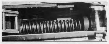
(above) The bolt is now driven forward by a single multi-strand spring, not the two nested recoil springs shown on this test prototype, wrapped around a guide tube and the buffer assembly. (below) The barrel recoil mechanism is wrapped around the Striker's barrel. There is also a finned barrel protector, made from an aluminum extrusion, over the barrel spring tube.
